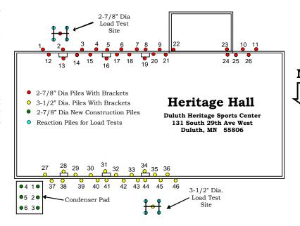
The project also called for six new construction helical piles to support a new concrete pad near the northeast corner of the structure. The pad will support a proposed condenser unit.
