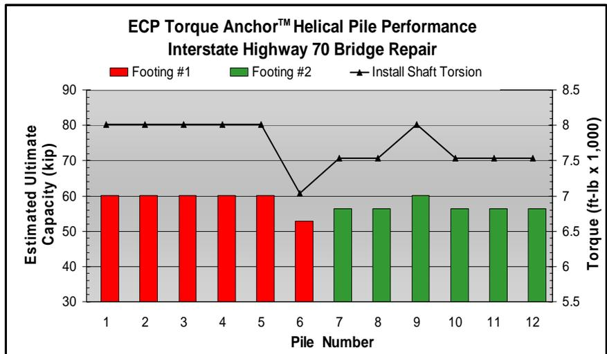
The piles were advanced into the soil using a 12,000 foot-pound hydraulic torque motor that was powered by a mini-excavator. A boulder was encountered during installation of one of the piles, which required a slight modification to the original pile layout plan.
