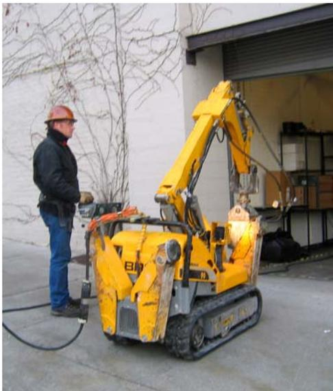
Photographs: At the top is a view showing the tight area of work in the emergency battery room. Access holes for the helical piles have been drilled in the floor. Unfortunately, obstructions required relocating several placements. At left is a view of the Brokk 90 Mobile Driller. The machine was fitted with an Eskridge 4K5 hydraulic gear motor that provided up to 4,500 foot-pounds of torque for the rotary installation of the piles.
